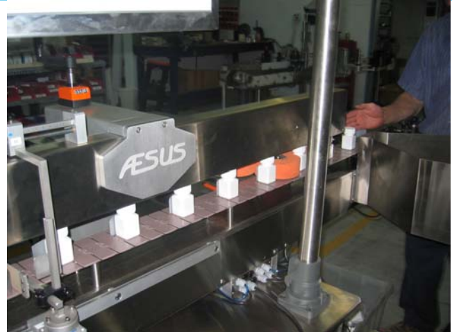
Adjust the height of the top hold down belt to press on the box gently.
