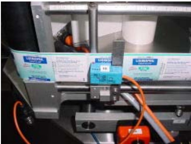
Adjust the label sensor to dispense the label appropriately.
