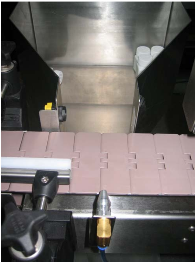
The positional adjustments to the wrap belt and the backup plate use simple locking handles.
