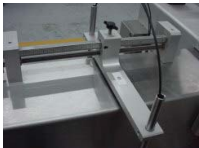
Adjust the product sensor by loosening the lock knob and turning the multi-turn screw.
