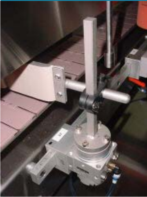
Adjust the position of the right and left wipers.
