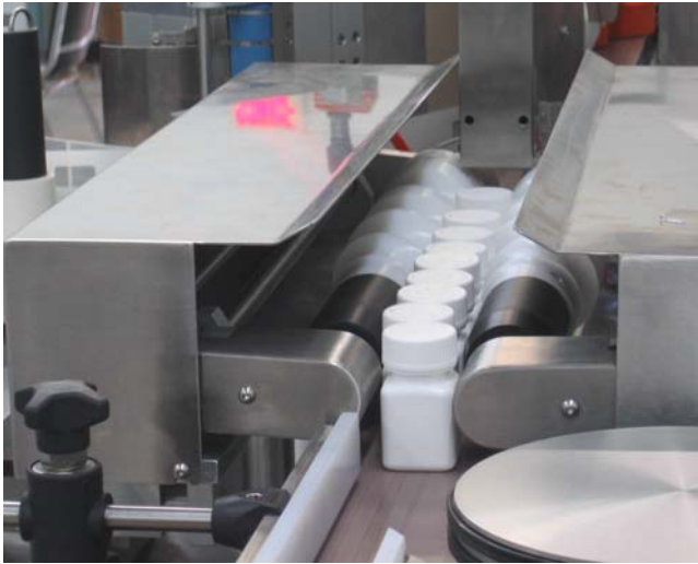
Adjust the height of the top hold down belt to press on the box gently.
