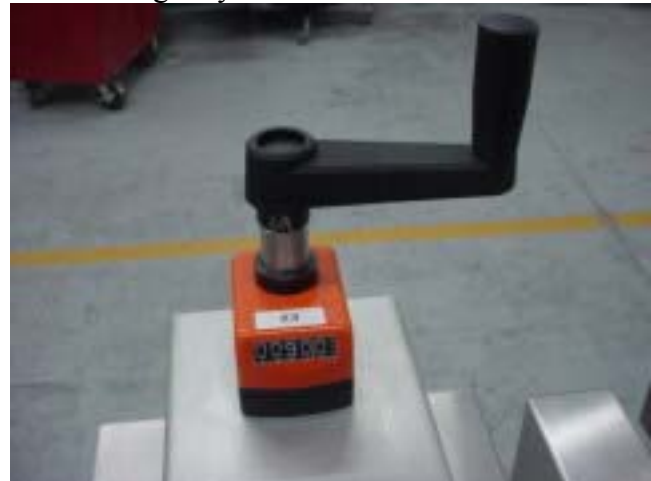
Adjust the height of the top hold down belt to press on the box gently.
