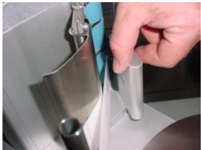
Adjust the label head vertically, adjust the tilt of the label, adjust the tilt in the other direction.
