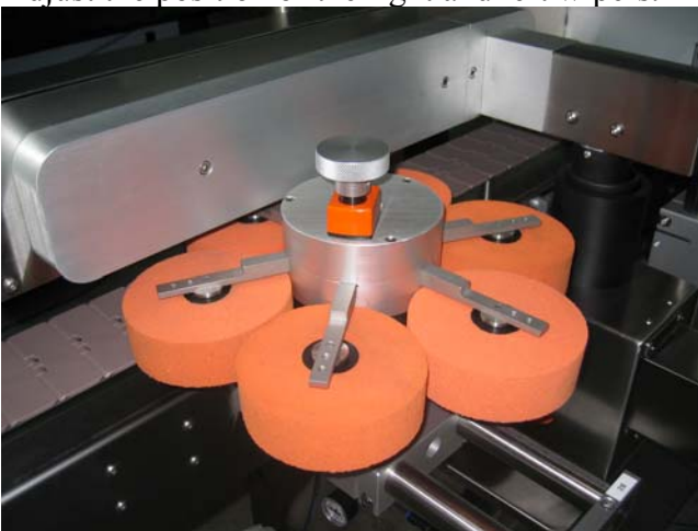
Adjust the rotary applicator using settings as given on the setup sheet for the bottle and style of labeling.
