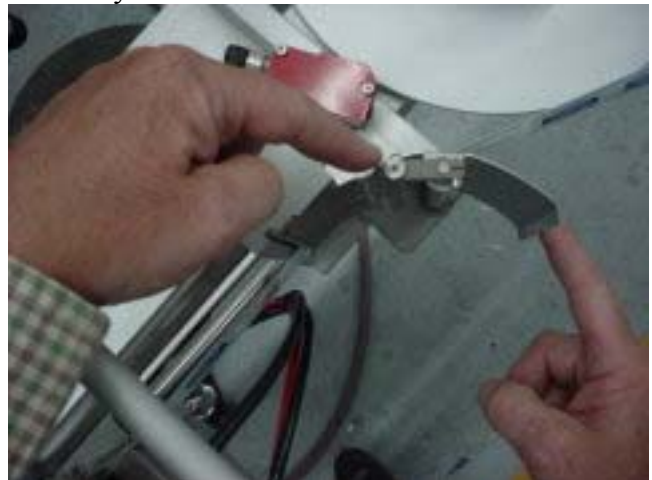
Pull the rear blade and lift the screw to snap back into tensioning mode.
