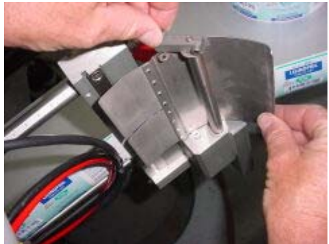
Adjust the tension device. Pull the small screw vertically to release.
