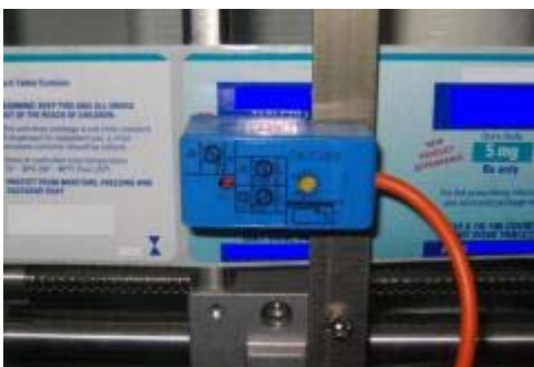
See Herma manual for full instructions on adjusting the label detection sensor. Different sensors are available.
