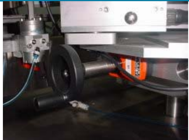
Adjust the label head horizontally.
